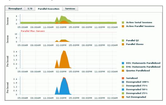
Figure 4-12 Monitoring Parallel Execution
