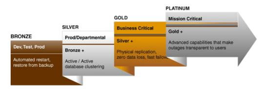
Each tier uses a different MAA reference architecture to deploy the optimal set of Oracle high availability capabilities that reliably achieve a given service level at the lowest cost and complexity. The tiers explicitly address all types of unplanned outages, including data corruption, component failure, and system and site outages, as well as planned outages due to maintenance, migrations, or other purposes.
