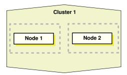
Using Figure 8-2 as an example, the following procedure explains how to add nodes to a cluster using cloning. In this procedure, you make a copy of the image (a clone) that you used to create Node 1, initially, to Node 2.
