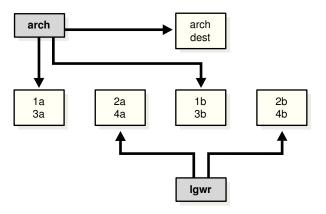
In this example, LGWR switches out of log group 1 (member 1a and 1b) and writes to log group 2 (2a and 2b). Concurrently, the archiver process reads from group 1 and writes to its archive destination. Note how the redo log files are isolated from contention.
