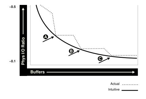
Figure 13-1 Physical I/O Ratio and Buffer Cache Size
