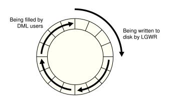
LGWR attempts to write fast enough to ensure that space is available in the redo log buffer for new entries, even if it is frequently accessed. Having a larger redo log buffer makes it more likely that there is space for new entries, and also enables LGWR to efficiently process redo records. On a system with large updates, if the redo log buffer is too small, LGWR will continuously flush redo to disk so that it remains two-thirds empty.
