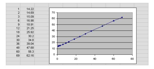
Figure 17-4 I/O Latency at Small I/O Load Levels
