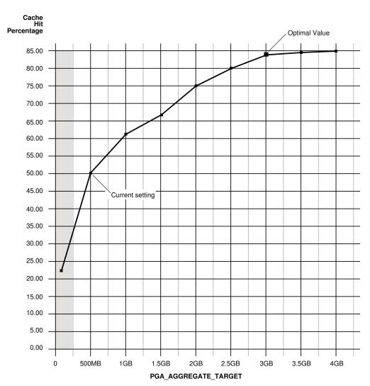
Figure 16-1 Graphical Representation of V\$PGA\_TARGET\_ADVICE
