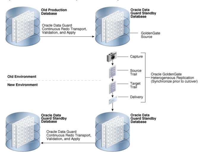
Figure 5-1 Oracle GoldenGate Configuration for Minimizing Planned Downtime
