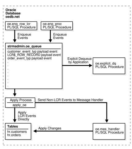
Figure 23-1 Example Oracle Streams Messaging Environment
