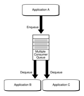
Figure 1-3 Communication Using a Multiconsumer Queue
